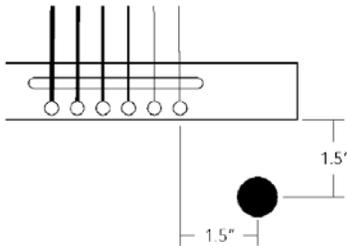
With freshly cleaned fingers, tear off a piece of the green putty (included), and spread it on the entire bottom surface of the pickup. The **AT-1** is rather lenient for placement, but we recommend you begin at the location above. Check the location by plugging in the pickup and listening. Should the position prove unsatisfactory, move the pickup in ¼" increments and re-test until you find the best position.
