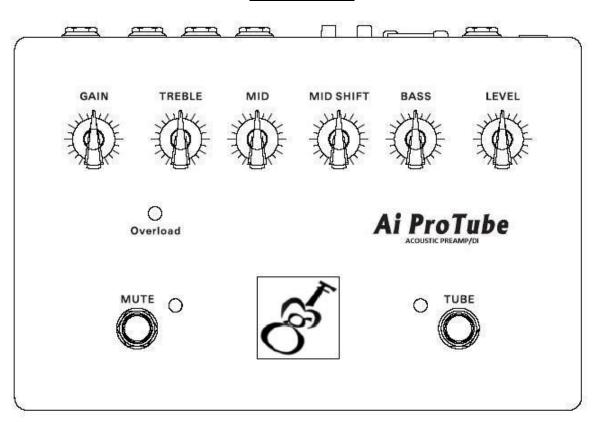
Power is supplied to the Ai ProTube via the 13VAC power jack, the tube window will illuminate when the unit is activated. (It will take a few seconds for the tube to warm up)
