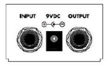
**9VDC** – This unit can run off 9V battery or you can connect a 9V adapter. The adapter must have a barrel connector with center negative. The battery may be left in or taken out when using an adapter. (To install or replace the 9V battery, loosen the screws on the bottom and remove the bottom plate. Be careful not to scratch the unit. Always remember to unplug your guitar cords from the pedal to conserve battery life.
