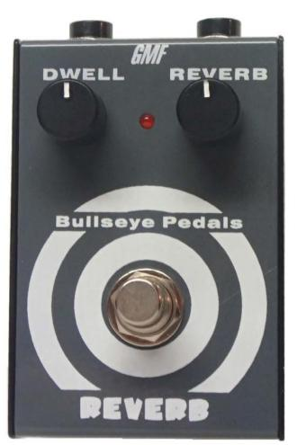
**DWELL** knob – This knob controls the decay of reverb. Rotating the knob clockwise will increase the decay time. **REVERB** knob – This knob controls the amount of reverb mixed with the dry signal. Rotating the knob clockwise will increase the amount of effect heard.
